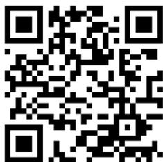
Print-and-cut jobs include an HP barcode as part of the print. This is read by the OPOS to find out where the cuts should be made. See [Read the HP barcode on page 24](#).
